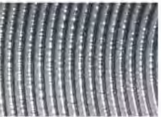
N11 R a 25 μm – AARH / CL 100 R t 102 μm
