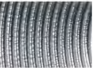
N12 R a 50 μm – AARH / CL 2000 R t 185 μm
